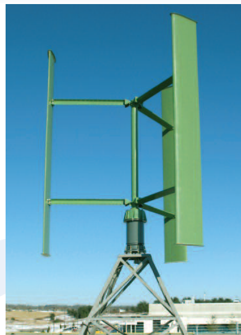
Cleanfield Energy's modular vertical axis wind turbine
