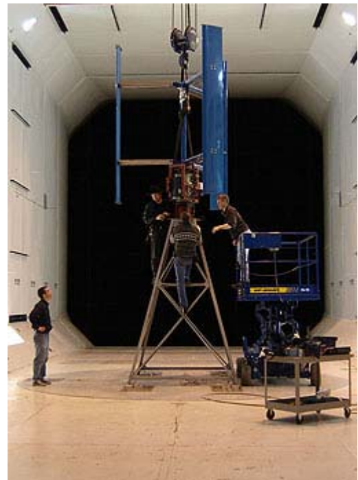
The Cleanfield V3.5 is a three-metre tall, vertical-axis wind turbine designed to provide electrical power for use by individual homes and businesses. Photo courtesy of Faculty of Engineering.
